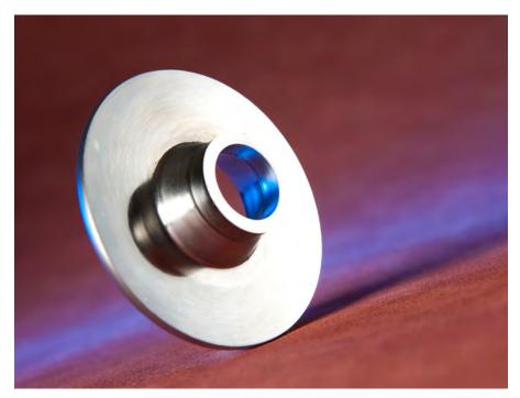
second operation procedures have been eliminated by the expanded capabilities of cold-heading equipment and tooling. Cold forming can also produce parts of a greater strength than machined parts. During machining, bar stock grain is interrupted, while cold-headed parts have a grain that follows the configuration of the part.
